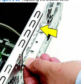
Figure 2-23 Replacing the bracket cover
